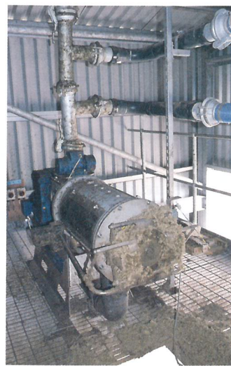
The new slurry separator produces the high fibre bedding.
